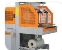
Efficient product loading using adjustable height entry conveyor
